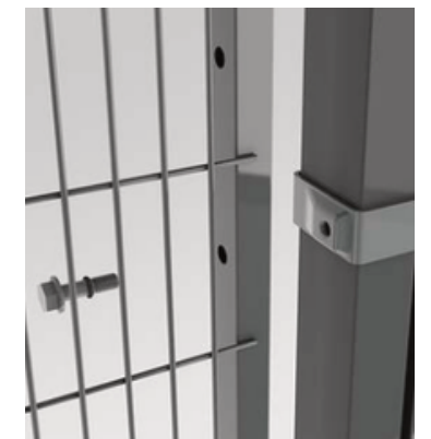
SMART FIX BRACKET Fixed in position with a bolt from the backside of the bracket. Move the bolt to the side position to create a corner.
